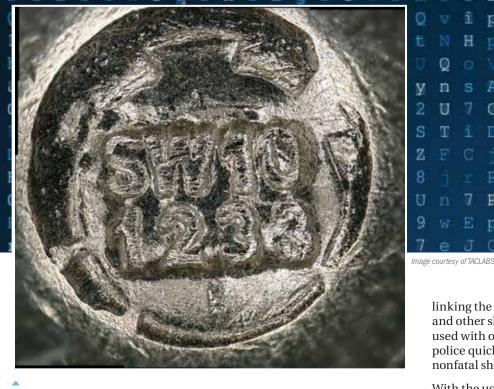
Magnified headstamp (150X magnification) of an expended cartridge casing with a microstamped primer impression created by a microstampequipped firing pin. Cartridge was fired from a 4006 S&W semiautomatic handgun.
