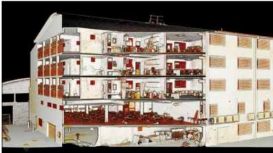
Above: With a pre and post event scan, users are able to determine relative change in environment down to 5mm (0.2").
