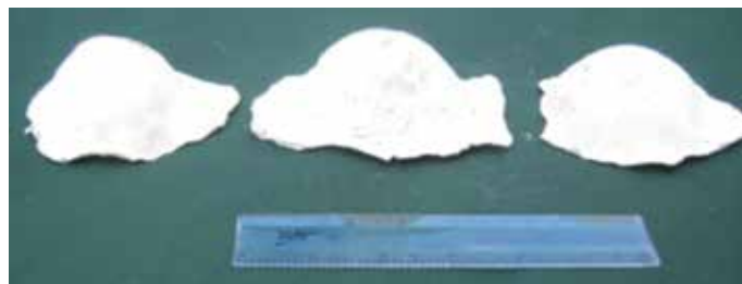
Figure 5: An example of the back deformations in the clay shown here with plaster of paris molds.
