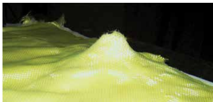
Figure 2: Photograph showing pencilin on the back-face of armor after testing.
