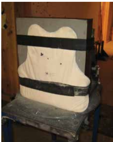
Figure 3: Plastilina block testing in accordance with HOSDB standards. The specified box size is slightly different in the NIJ standard. However, the difference is unlikely to affect the results obtained during testing.
