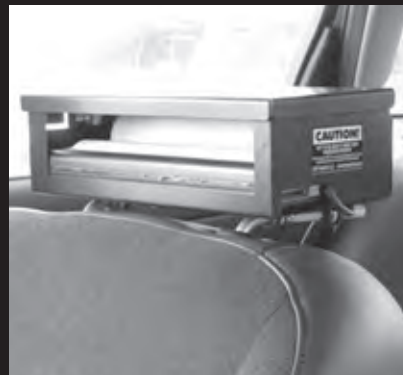
Headrest Mount for Pentax Pocket Jet Printer
