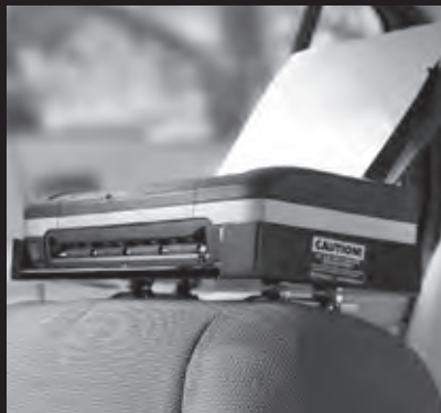
Headrest Mount for HP470 Deskjet Printer
