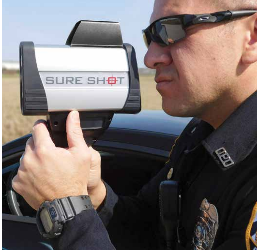
The Sure Shot radar device has a touchscreen and can record up to 500 shots. (Photo courtesy of MPH Industries, Inc.)
